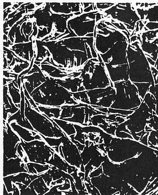
3. Cotton linters fibers. SEM, magnified 115 times.
