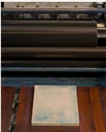
▶ Lino block is laid in press bed before printing.
