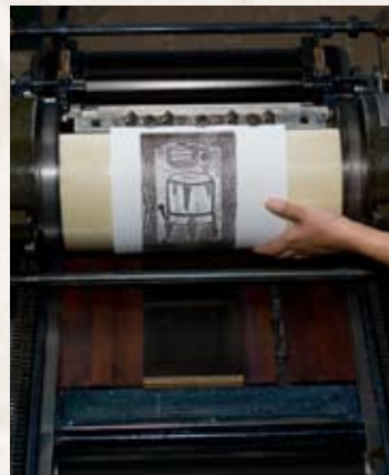
▶ Run matrix through press underneath paper
