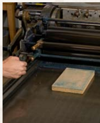
▶ Adjust roller height to accommodate for matrix
