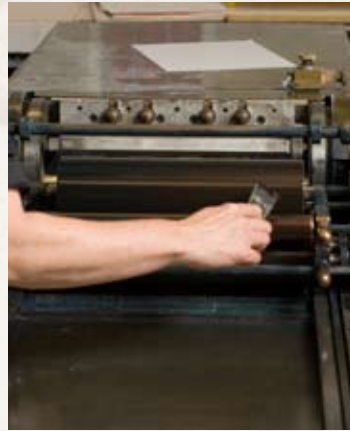
▶ Ink is applied by hand to rollers on press
