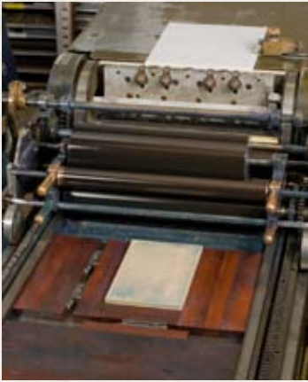
▶ Lino block is laid in press bed
