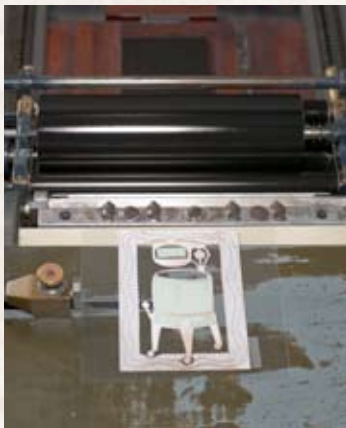
▶ Matrix must be registered underneath paper
